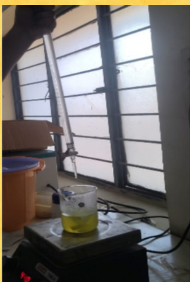
Figure 1.8 : Synthesis of PTSA doped Polyaniline
